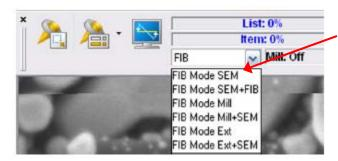
8. Referring to the SmartSEM GUI, select FIB mode SEM in the FIB Mode selection window
