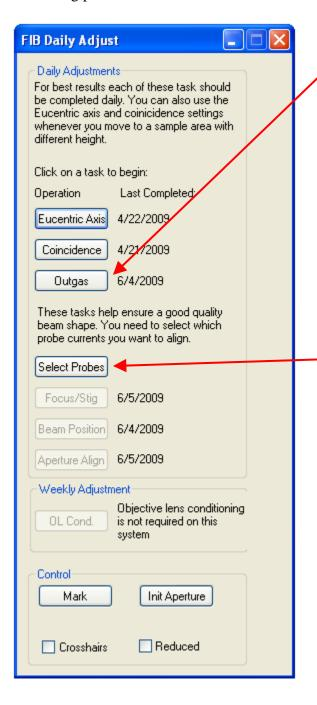
As previously mentioned, perform the precursor outgas procedure by clicking on the "Outgas" button. This starts a macro, which allows you to select a precursor to outgas and execute the procedure. If a precursor has NOT been recently out-gassed, an asterisk will appear next to the precursor's name. In this case, carry out the procedure. Otherwise, skip Outgas.
