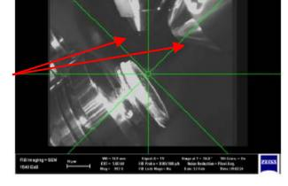
travel motor speed is linked to magnification. The lower the magnification, the faster the motion. As the image begins to come back into focus, increase magnification and continue moving the stage up until the sample is in focus at 5 mm WD
