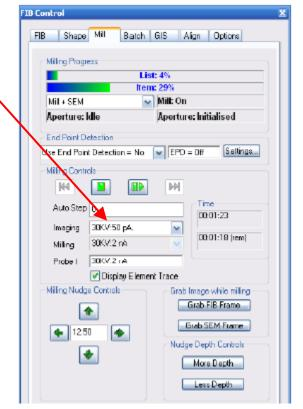
Using a probe current of (or just under) 5 pA/μm<sup>2</sup> of deposition area
