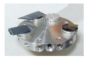
2. Mount sample holder onto dovetail with threads facing rod tip **Do not attach rod to holder at this time!**
