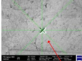
13. Click view on the menu bar, and select "Crosshairs" from the list. This will display a fixed set of graphics used as reference to adjust tilt-eucentricity and coincidence between the SEM and FIB
