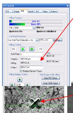
24. In order to reduce the amount of material removed during FIB imaging, select a low FIB imaging probe current from the Mill tab of the FIB Control panel. Use a probe current ≤ 80 pA
